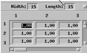
The spatial filter process provides several predefined filter window sizes up to 11 x 11 cells. You can create a larger filter window by typing new values in the Width and Length text boxes on the Kernel tabbed panel.
