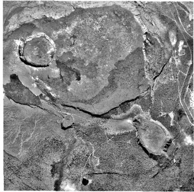
The LACE filter process adjusts the brightness of input cells by calculating a gain coefficient for each cell based on the local standard deviation. The Gain Limit parameter sets an upper limit on the value of this coefficient and on the degree of contrast enhancement that results in a given area.
